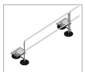
HR1002 – 2 Bar Safety Rail – Is designed specifically for use on rooftop without adhesive, roof penetrations, flashings or damage to roofing system. Modular Safety Rail system designed to be easily installed anywhere safety barriers are needed. Posts connect using hinged designed for versatile layout and easy assembly. Use ballast weight if additional stability is needed.
